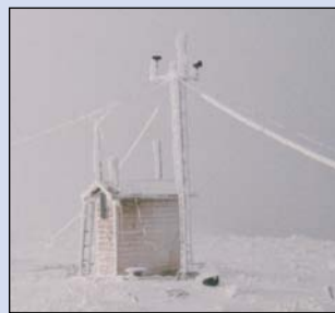
Rime ice on monitoring equipment on Haeckel Hill, 1994. Only heated instruments stay clear of ice.
